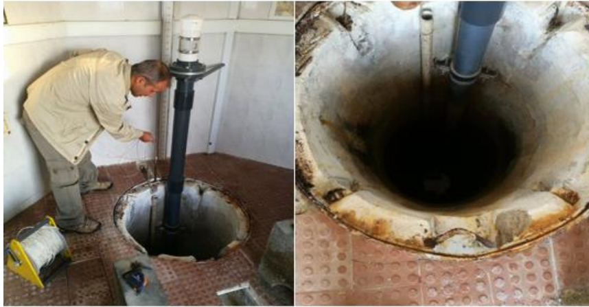
Figure 2: Tide gauge (Lagos). Left: Placement of the transducer (Level TROLL 400) in the well of Lagos national tide gauge. Right: Submerged transducer (Level TROLL 400) placed inside the well.
